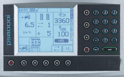
The RDS Artemis removes the need for a mechanically driven land wheel by operating the metering unit with an electric motor maintaining its speed proportional to forward speed.
