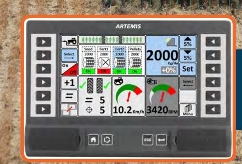
A multi-channel electric drive system providing the control and monitoring requirements of the modern seed drill.
