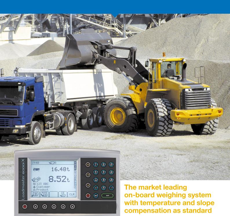
The RDS Loadmaster 8000iX is a highly accurate, dual sensor, temperature and slope compensating on-board weighing system for larger loaders that can help increase loading efficiency, cut vehicle movements on site increasing safety and ensure lorries are correctly loaded first time.
